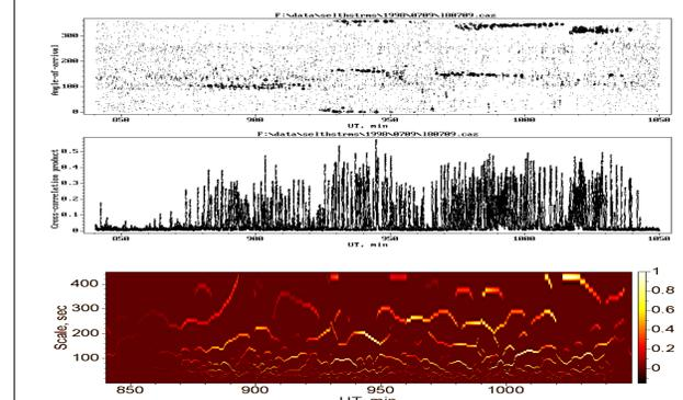
Fig 9: Lycksele, 1998-07-09 14:00 – 17:30 UT. Top graph: angle-of-arrival, middle graph: cross-correlation product, bottom graph: dominating time scales (wavelet skeleton spectrum).
